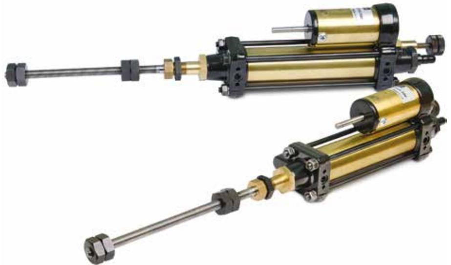
Hydrochecks are precision built self contained hydraulic control units designed to smooth out pneumatic cylinder movements over any distance within their own stroke length, up to 450 mm.
