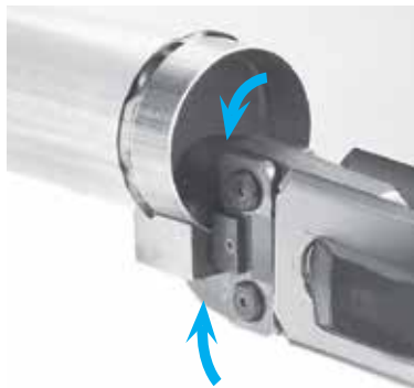
Release the jaws. Press the trigger and crimp the tube until a 'snap' sound is heard.
