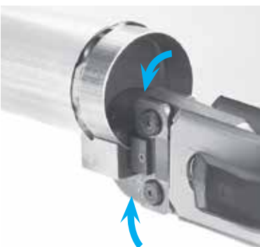
Repeat the operation until the required minimum number of lugs for each diameter is achieved.
