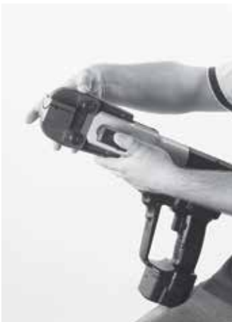
Lock in position by closing the retaining pin.
