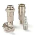
Safety coupling with UltraFlo-Valve for optimum flow and low pressure drop. The series stands out for its robust design (steel sleeve) and long service life even with the harshest use. Additional safety locking system. This safety lock prevents unintentional disconnection. To disconnect, the plug must first be pushed further into the coupling before it can be unlocked. The brass version has been developed specifically for use with water in the pressure range up to 35 bar.
