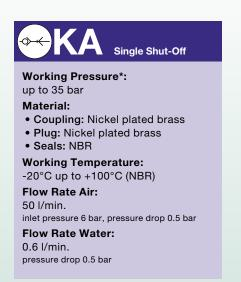
\* maximum static working pressure with design factor 4 to 1.
