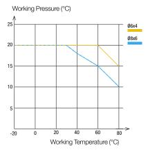
To calculate burst pressure, the values in these graphs should be multiplied by 3.
