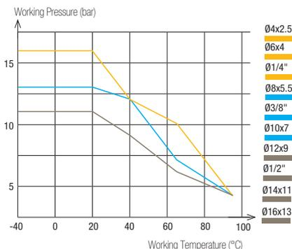
To calculate burst pressure, the values in these graphs should be multiplied by 3.
